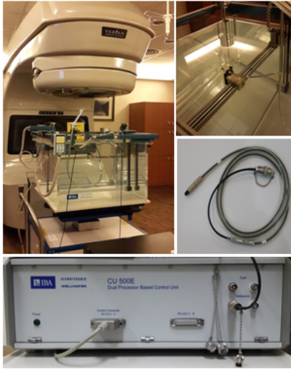
Fig. 2. Setup image and equipment for measurement the PDD.
