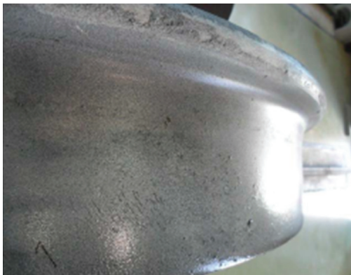
Fig. 3 Tread of wheel damper (before test)
