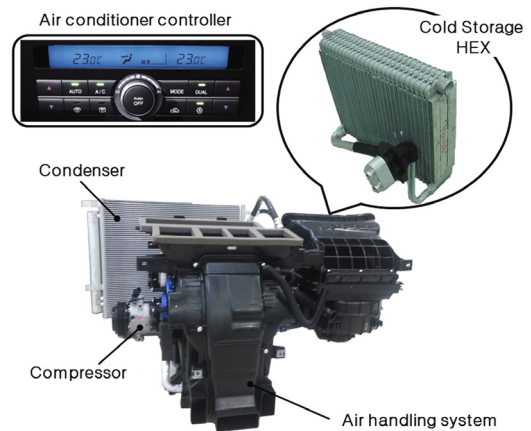
Fig. 2 Configuration of cold storage system and controller
