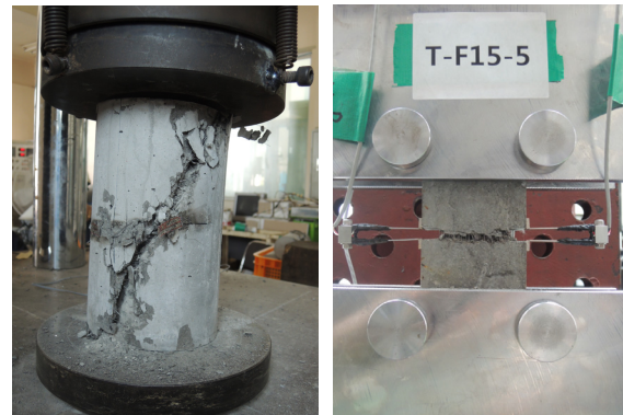
<Fig. 1> (Left) Compressive strength test and (Right) Direct Tensile strength test of UHPFRC
