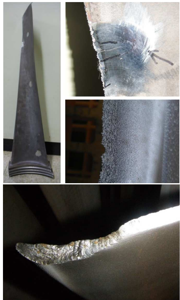
Fig. 1 Defect detected in airfoil's leading edge
