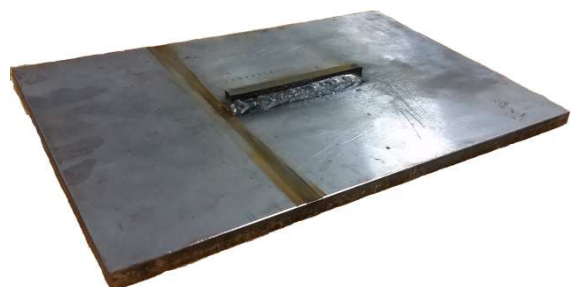
(a) 30mm cutting by wire cutting machine(10mm of rib remained)
