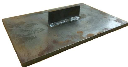
Fig. 1 Fillet weldment(rib height 40mm)
