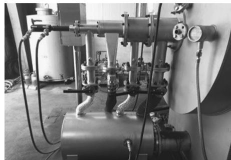
Fig. 4. Picture of the Pet-coke burner.
