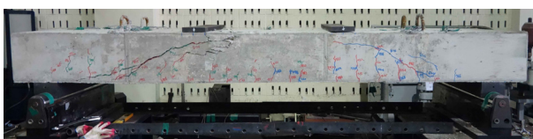
Fig. 9 Shear failure mode(WF240-A2)
