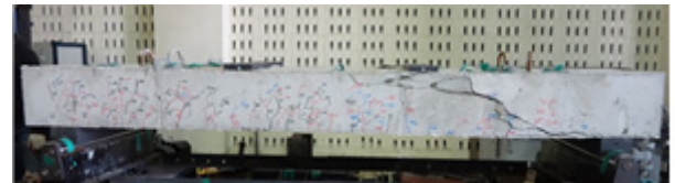
Fig. 6 Shear compression failure(WS240-2)
