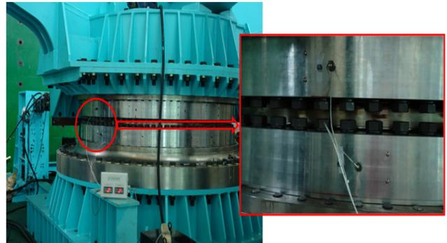
Fig. 10 Raceway temperature measurement using thermocouple
