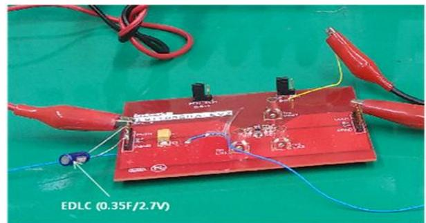
Fig. 6. ISL9110A test board
