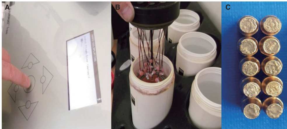
Fig. 2. (A) Adjustment of the device for Electroforming process, (B) Placement of dies into the loading head of device and (C) Galvano copings obtained after electroforming.
