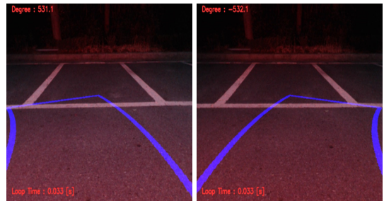
Fig. 22. Parking guideline according to handle steering angle
