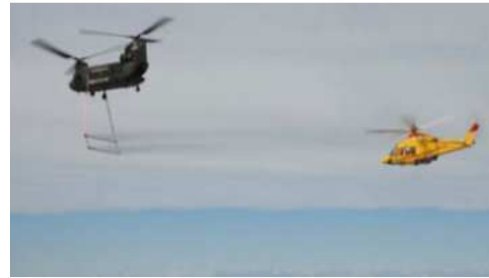
Fig. 3. HISS system for artificial icing flight test
