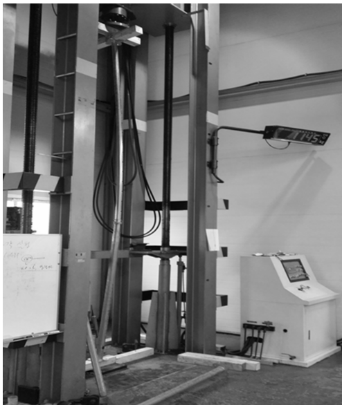
Fig. 6. The buckling test of pipe support.
