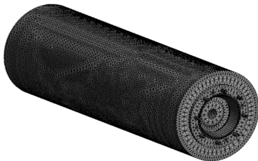
Fig. 2. FEM mesh for analyzing stress and deformation of a cylindrical roller.
