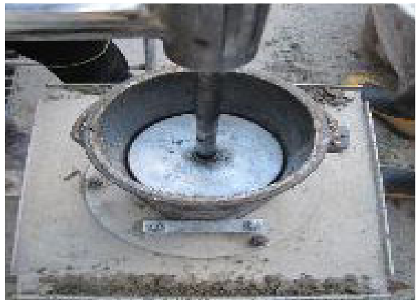
(b) Making Cylinder Molds Using a Vibrating Table
