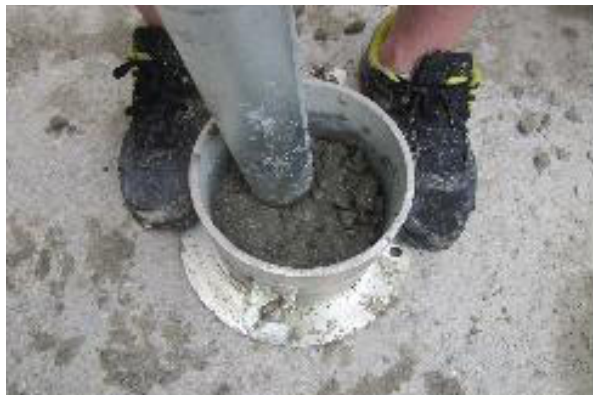
Fig. 6 Modified Proctor Test According to ASTM D1157
