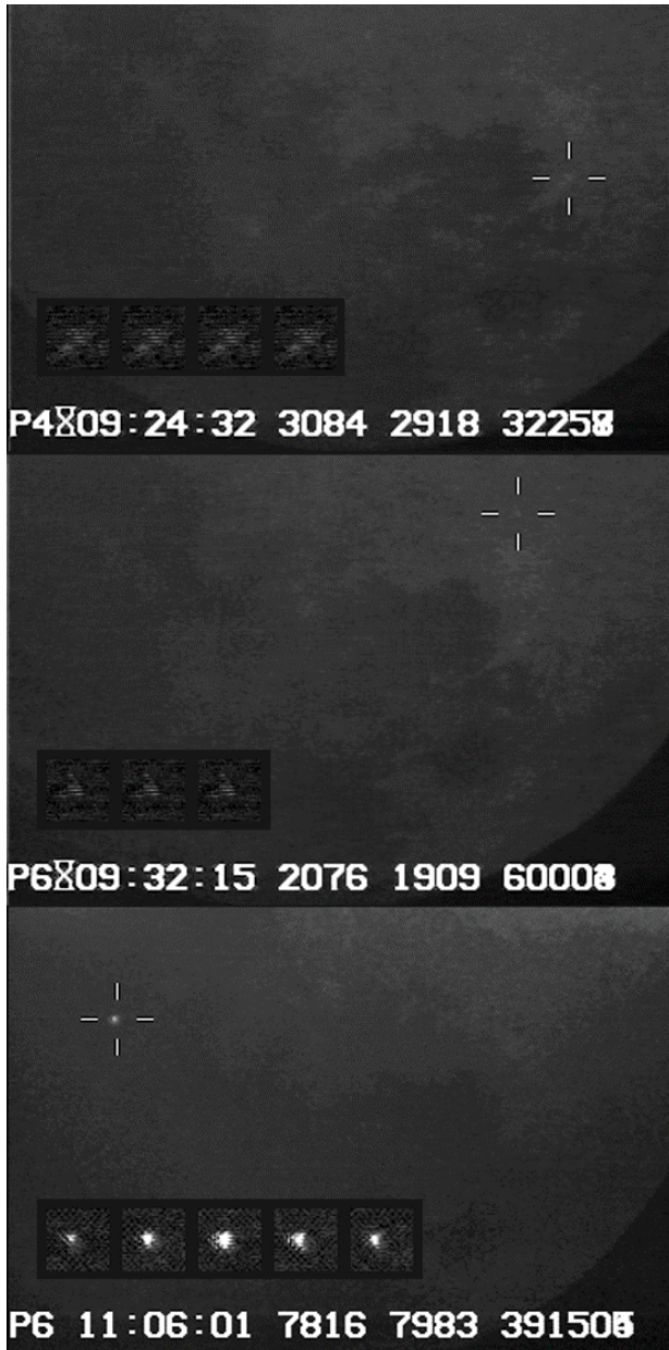
Fig. 3. The impact flash candidates observed at Jan. 4, 2014, 9:24:32 UT (top), 9:32:15 UT (middle), and Feb. 3, 2014, 11:06:01 UT (bottom). The flash position is marked with a cross and a sequence of frames is shown in the lower part. The GPS time (UT) and frame numbers of the image are displayed using white letters.
