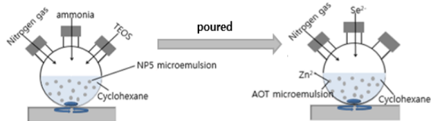
Figure 1. Schematic of synthetic method for silica-encapsulated ZnSe quantum dots.
