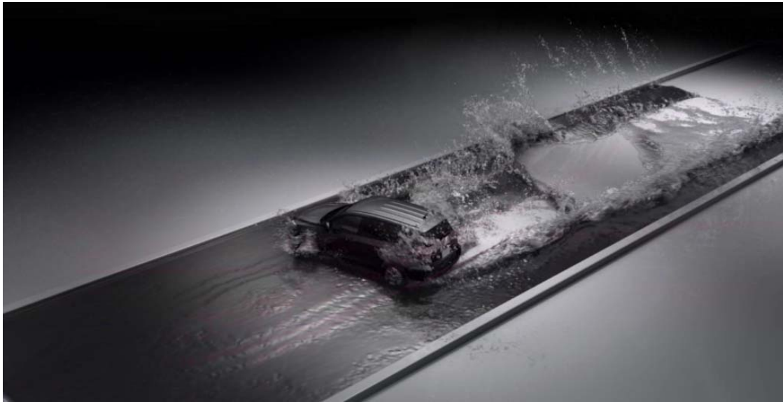
Fig. 2 Free surface problem solved by Particleworks using MPS method
