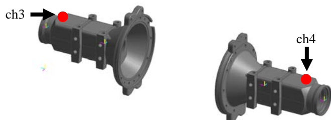
Fig. 4 Measuring point of acceleration at rear axle
