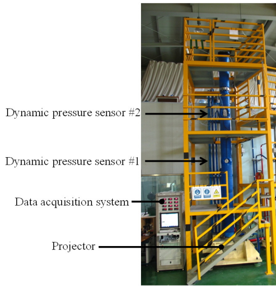
Fig. 2. Pulse tube for measurement of transmission loss.
