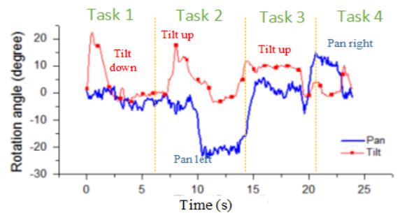
Fig. 14 The pan/tilt angular tracking by IMU sensor
