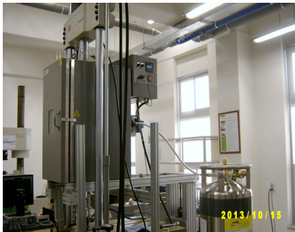
Fig. 5. Tensile-fracture load test (GFRP coupon specimens at sea water temperature)
