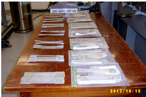
Fig. 3. Coupon specimen for tensile tests
