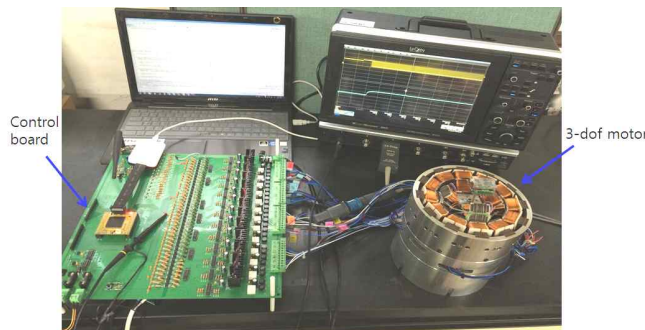
Fig. 11. PI current control experiment of double excited 3-DOF motor.
