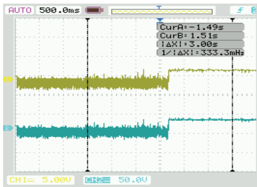
Fig. 9. Digital signal control output voltage and current waveforms.
