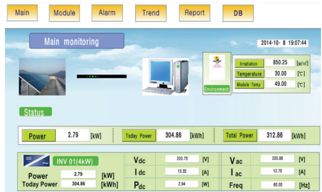
Fig. 7. Monitoring function of state diagnosis system
