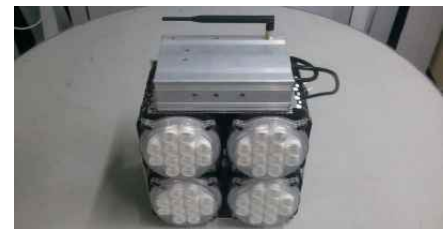
(b) Single SMPS integrated with wireless communication module
