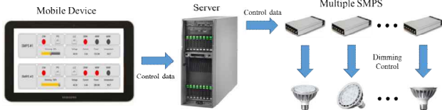
(a) Data flow process for the multiple SMPS control
