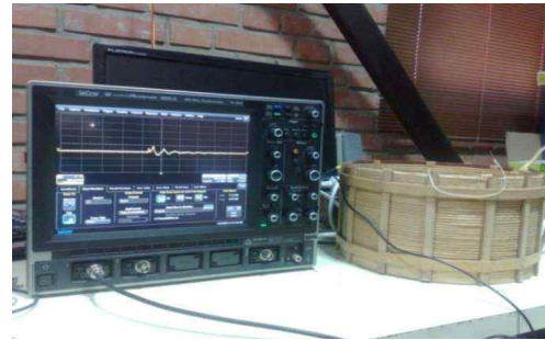
Fig. 21. The tested distribution 20 kV transformer winding
