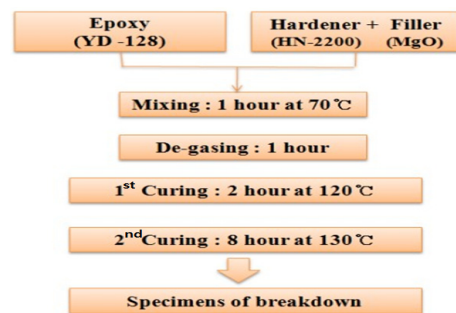
Fig. 2. Block diagram of specimens manufacturing process.
