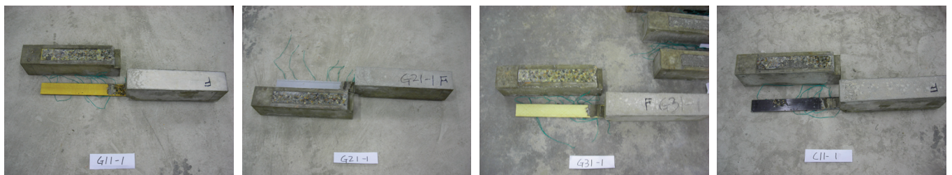
Fig. 5 Failure Shape of GF11, GF21, GF31 and CF11- NOCON
