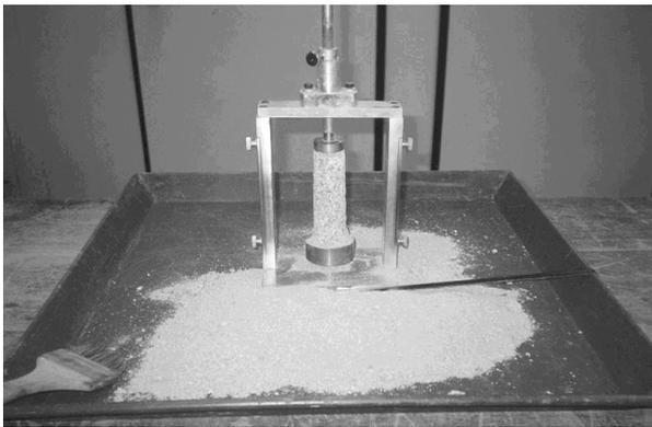
Photo 1 Trimming process of undisturbed samples
