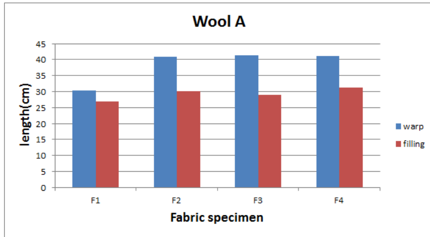
Figure 5. Stiffness of fabrics treated with Synthappret R-BAP, Wool A (D : Measured specimen length, cm)
