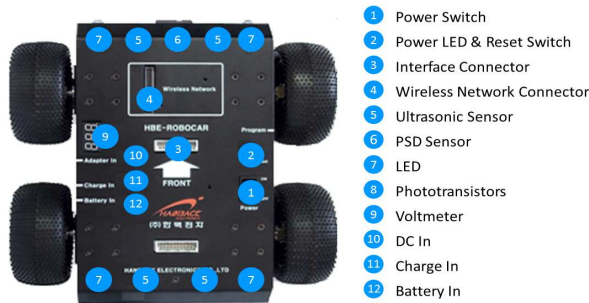
Fig. 7 Mobile robot hardware and sensor (RoboCAR 28 )
