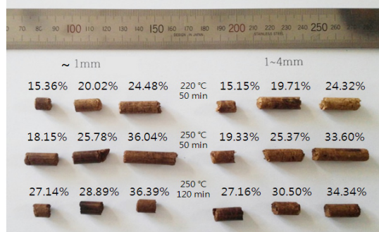
Photo 1. Pellet prepared with torrefied larch on different condition at 120°C of die temperature.
