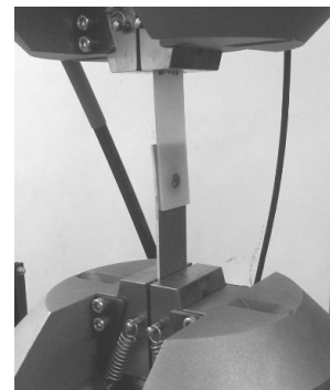
Fig. 10 Shear testing for self-pierce riveted zone of GFRP and Al5052 sheets
