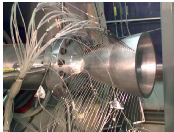
Fig. 5. Dual-bell nozzle during testing at the NASA[12]
