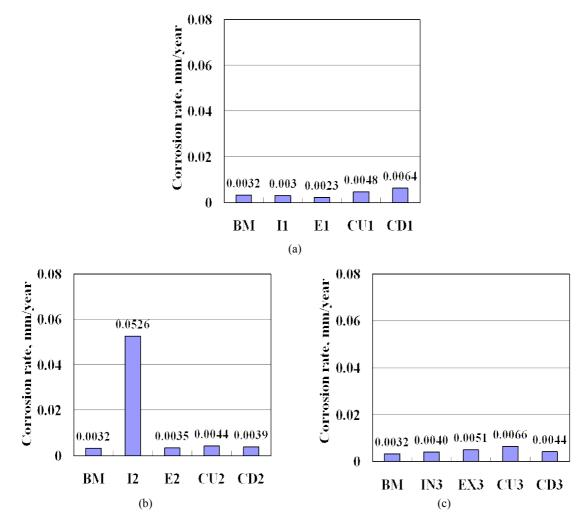
Fig. 7. Corrosion rate for base metal and bended areas of ASME SA106 Gr. C carbon steel in deaerated 5,700 ppm boric acid  $200^{\circ}$ C for 100 hours: (a) transition start, (b) bend and (c) transition end.
