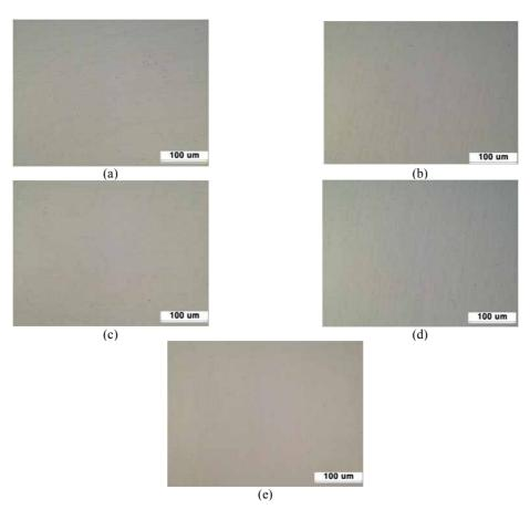
Fig. 2. Inspection of non-metallic inclusion on base metal and bended areas of ASME SA106 Gr. C carbon steel: (a) I1, (b) E1, (c) CU1, (d) CD2 and (e) base metal.
