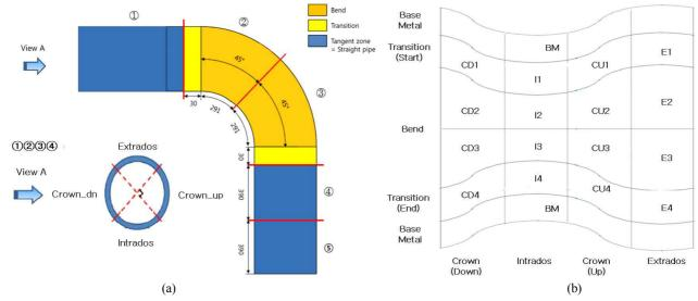
Fig. 1. Schematic diagram of (a) ASME SA106 Gr. C carbon steel bent pipe and (b) identification symbols.
