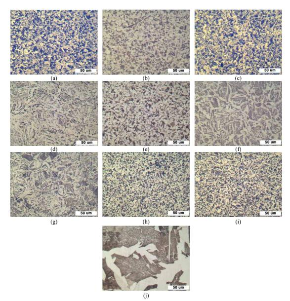
Fig. 3. Optical microstructures of base metal and bended areas of ASME SA106 Gr. C carbon steel: (a) I1, (b) E1, (c) CU1, (d) I2, (e) E2, (f) CU2, (g) I3, (h) E3, (i) CU3 and (j) base metal.
