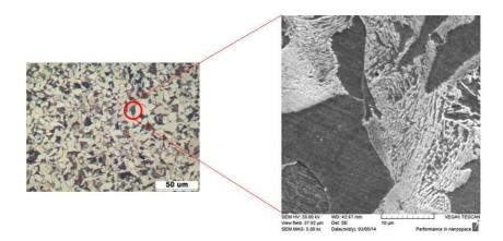
Fig. 5. Optical and SEM images on extrados areas (E2) of bended pipe of ASME SA106 Gr. C carbon steel.
