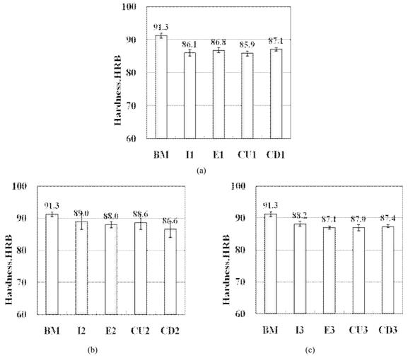
Fig. 6. Rockwell hardness of base metal and bended areas of ASME SA106 Gr. C carbon steel: (a) transition start, (b) bend and (c) transition end.
