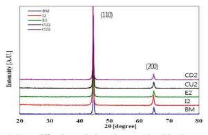
Fig. 4. X-ray diffraction analysis on base metal and bend areas of ASME SA106 Gr. C carbon steel.
