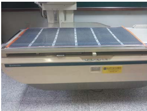
Fig. 5. carbon heating elements diagnosis table and X-ray equipment.
