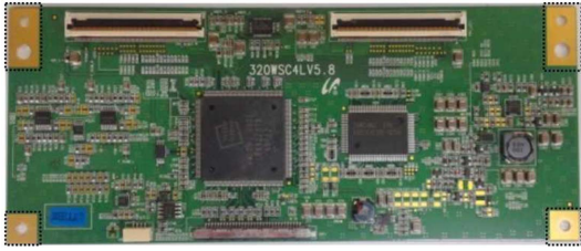
Fig. 2. PCB fabricated by ENEPIG process.
