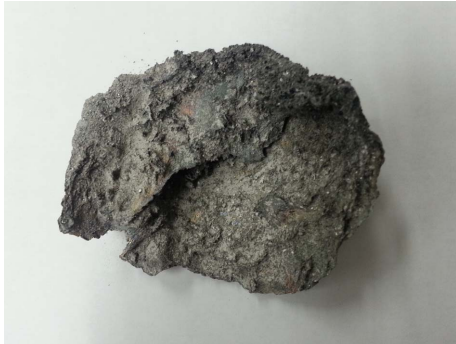
Fig. 8. Photo of hard head after slag reduction.
