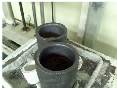
Fig. 2. Photo of the carbon crucible for smelting.
