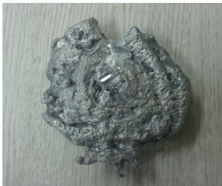
Fig. 6. Photo of crude Tin after the 1 st smelting.
