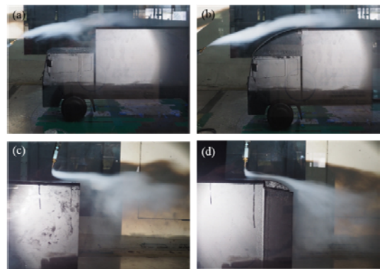
Fig. 8. Visualized flow around the cab-roof fairing and boat tail of the 5ton truck model.
