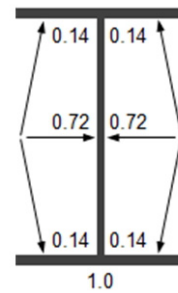
Fig. 11. View factor to consider the shadow effect of H section in the numerical analysis
