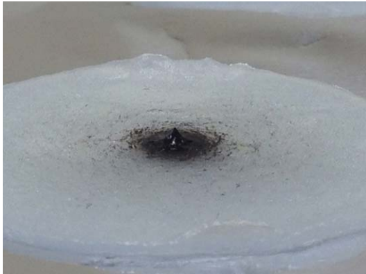
Fig. 1. One week accumulation of aerosol larger than 2.5 \mu\text{m} on the WINS Impactor surface.
