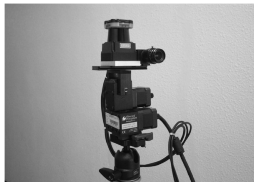
Fig. 7. LRF-camera Setup used in the Experiment
