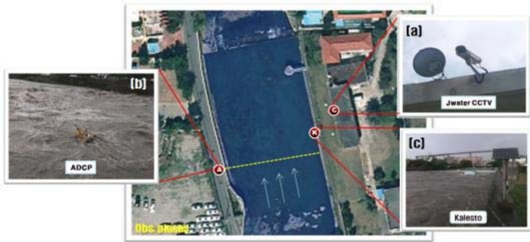
Fig. 3. Observation point and method: a) Disaster monitoring CCTV system; b) Acoustic Doppler Current Profiler; c) Kalesto.
