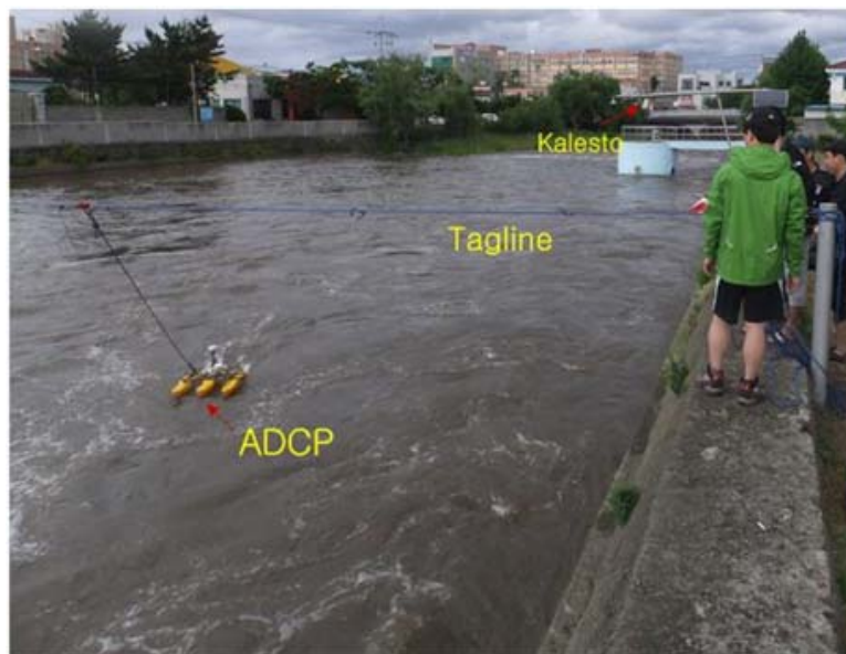
Fig. 3. Velocity and discharge measurements of flood conditions using ADCP dragged along the installed tagline across the given cross-section.
