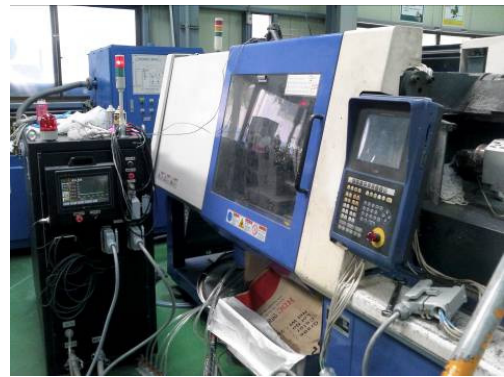
[Fig. 2] Injection molding device for mold temperature control
