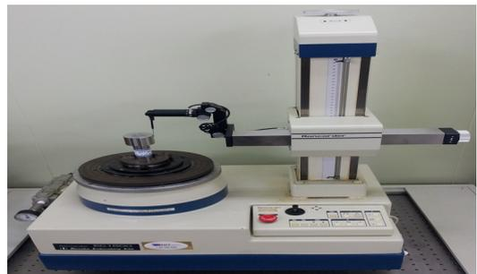
[Fig. 8] Circularity testing machine(EC1800)
