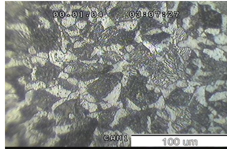
[Fig. 3] Base metal zone of SM45C
